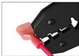
04. Insert the wire into the spade, and crimp it down to secure the wire
