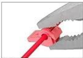
03. Squeeze the connector together until it locks
